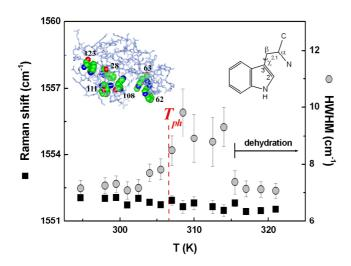
Temperature dependences of frequency and bandwidth (HWHM is a half-width at half-maximum) of 1613 cm<sup>-1</sup> band originating from C-C stretching vibrations within the aromatic ring of Tyr groups. The values of Raman shift are shown by black squares, the values of HWHM – by gray circles. The insert in the figure shows locations of Tyr residues in lysozyme molecule.
