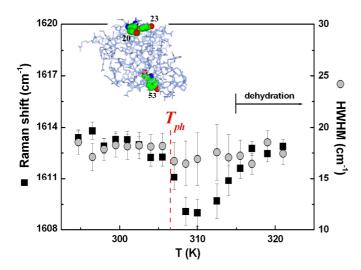
Temperature evolution of 694 cm<sup>-1</sup> band originating from C–S stretching vibrations of Met residues of lysozyme molecule: (a) Raman spectrum in the vicinity of the band and its fitting, the insert shows locations of Met residues in lysozyme molecule; (b) temperature dependencies of frequency and bandwidth (HWHM is a half-width at half-maximum) of the band. The values of Raman shift are shown by black squares, the values of HWHM – by gray circles.
