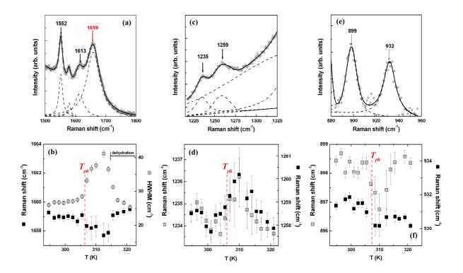
Temperature dependences of frequency and bandwidth (HWHM is a half-width at half-maximum) of  $1552 \text{ cm}^{-1}$  band arising from  $C_2$ = $C_3$  stretching vibrations of Trp indole rings. The values of Raman shift are shown by black squares, the values of HWHM – by gray circles. The inserts in the figure show locations of Trp residues in lysozyme molecule and structural formula of Trp residue.
